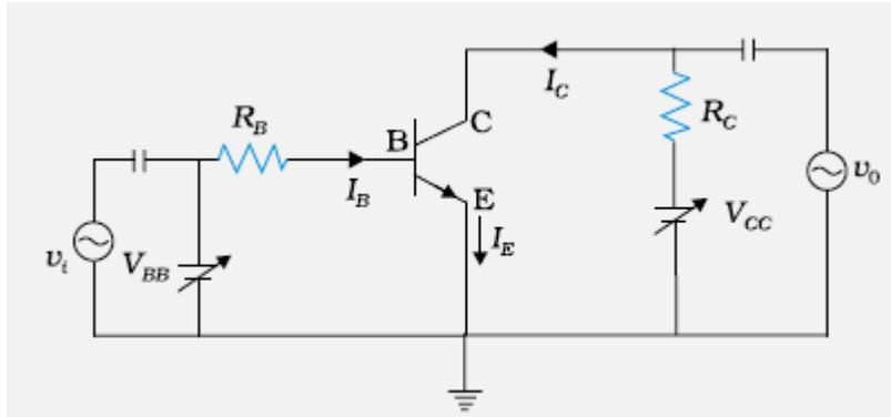
The input signal, connected between the emitter and base, along with the forward bias, causes corresponding large changes in output voltage across R.
